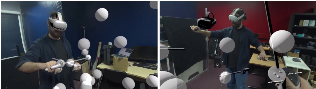
Fig. 4.1 First-person view of a user manipulating their viewpoint, either coupled (left) or decoupled (right), the other's point of view is represented by a virtual headset.
