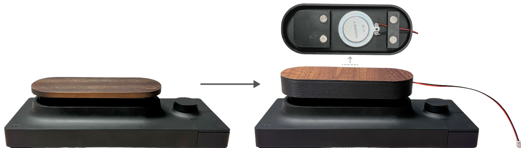
Fig. 3.4 Touché faceplate redesign with 3D printed part and voice coil embedded.
