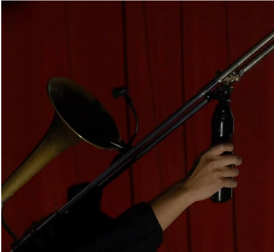
Fig. 3.6 An early implementation of the mubone using a Wii remote.
