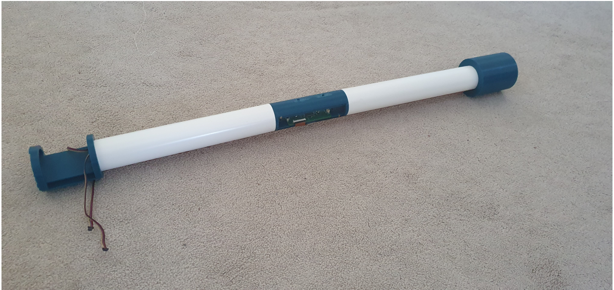
Fig. 5.10 Partially assembled Soprano T-Stick 5GW, the touch board bed, and endcap are glued onto the plastic pipe.
