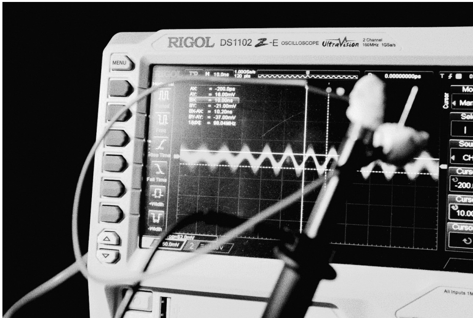
Figure 4.30: Breadboard wire picks up 82 mV peak-to-peak interference at around 98 MHz.
