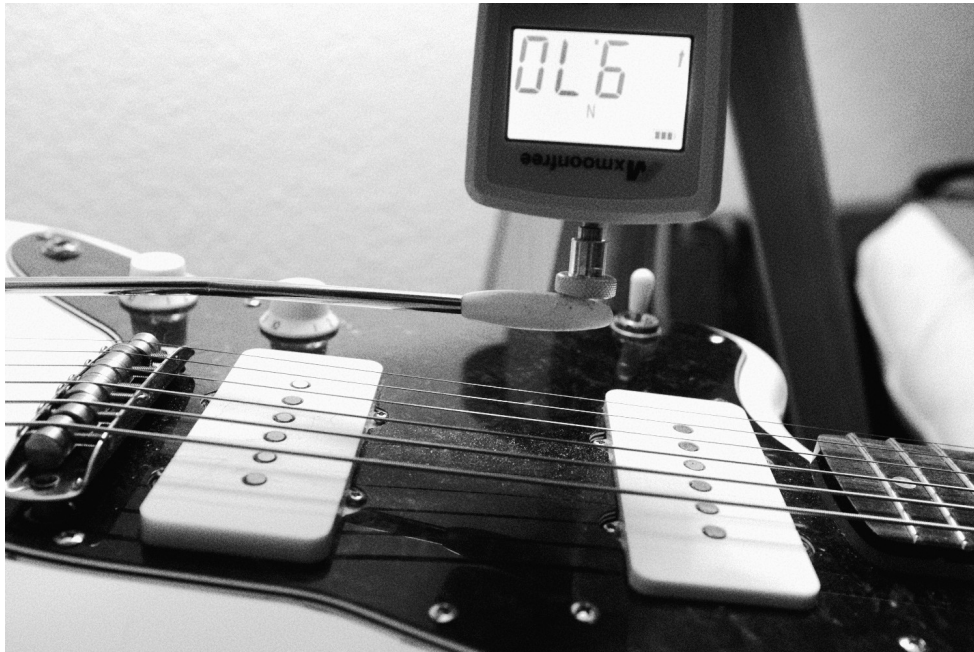
Figure 2.11: Measuring setup for the force response. The gauge is pushed to the maximum.
