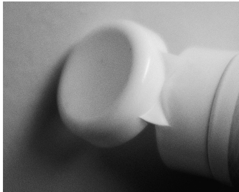
Figure 4.4: Compliant mechanisms are used on face cleanser bottles to provide a spring-like closing force when the cap is half open to prevent leaking.
