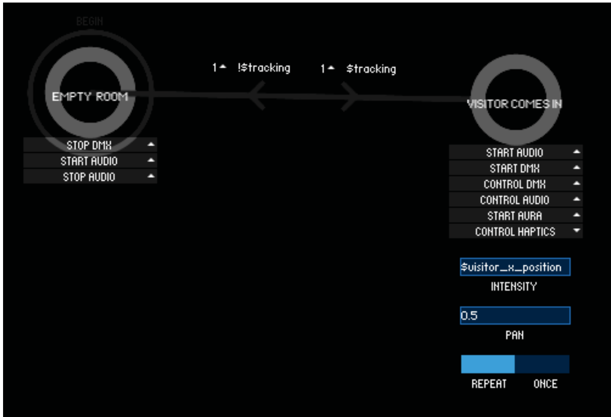
Fig. 5.1 ZenStates allows users to quickly prototype interactive environments by directly manipulating States connected together via logical Transitions . Tasks add concrete actions to states and can be fine-tuned via high-level parameters (e.g. ‘intensity’ and ‘pan’). Blackboard global variables (prefixed with the ‘$’ sign) can enrich tasks and transitions. © 2018 IEEE.
