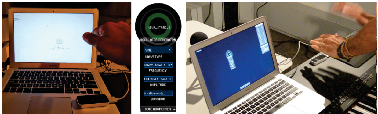
Fig. 6.6 We can quickly modify our theremin example to make it more realistic (image (c)) in two steps. First, we use the Leap Motion sensor and an OSC converter software (image(a)). Second, we modify our previous example from Figure 6.3 to match image (b): that is, we replace ‘mouseX’ and ‘mouseY’ variables by the incoming-OSC blackboard variables (‘left_hand_z_0’ and ‘right_hand_z_0’) and add a note augmenter to eliminate the need of key pressings.
