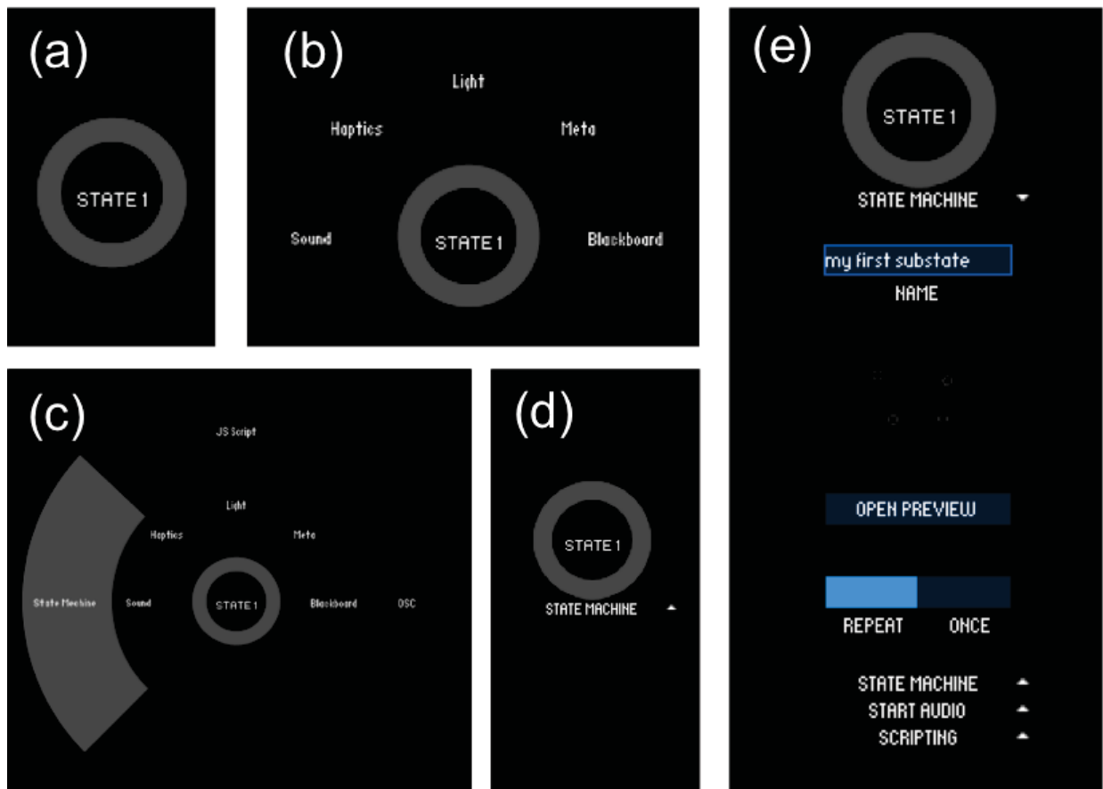
Fig. 5.3 Tasks inside states are reified with a contextual pie menu, as shown in the sequence above—(a), (b), (c), and (d). High-level parameters related to each task can be found by clicking on the task—as shown in (e). © 2018 IEEE.
