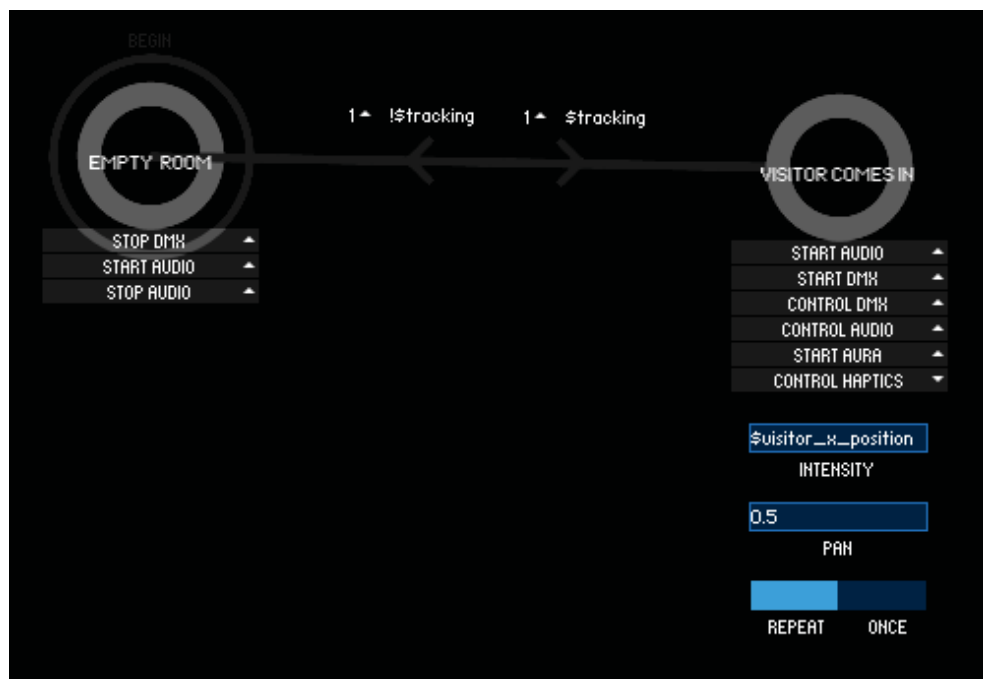
Fig. 4.5 ZenStates allows users to prototype behavioral responsive environments by directly manipulating States connected together via logical Transitions . Tasks add concrete actions to states, and can be fine-tuned via high level parameters (e.g., ‘intensity’ and ‘pan’) Blackboard global variables (prefixed with the ‘$’ sign) can enrich tasks and transitions.
