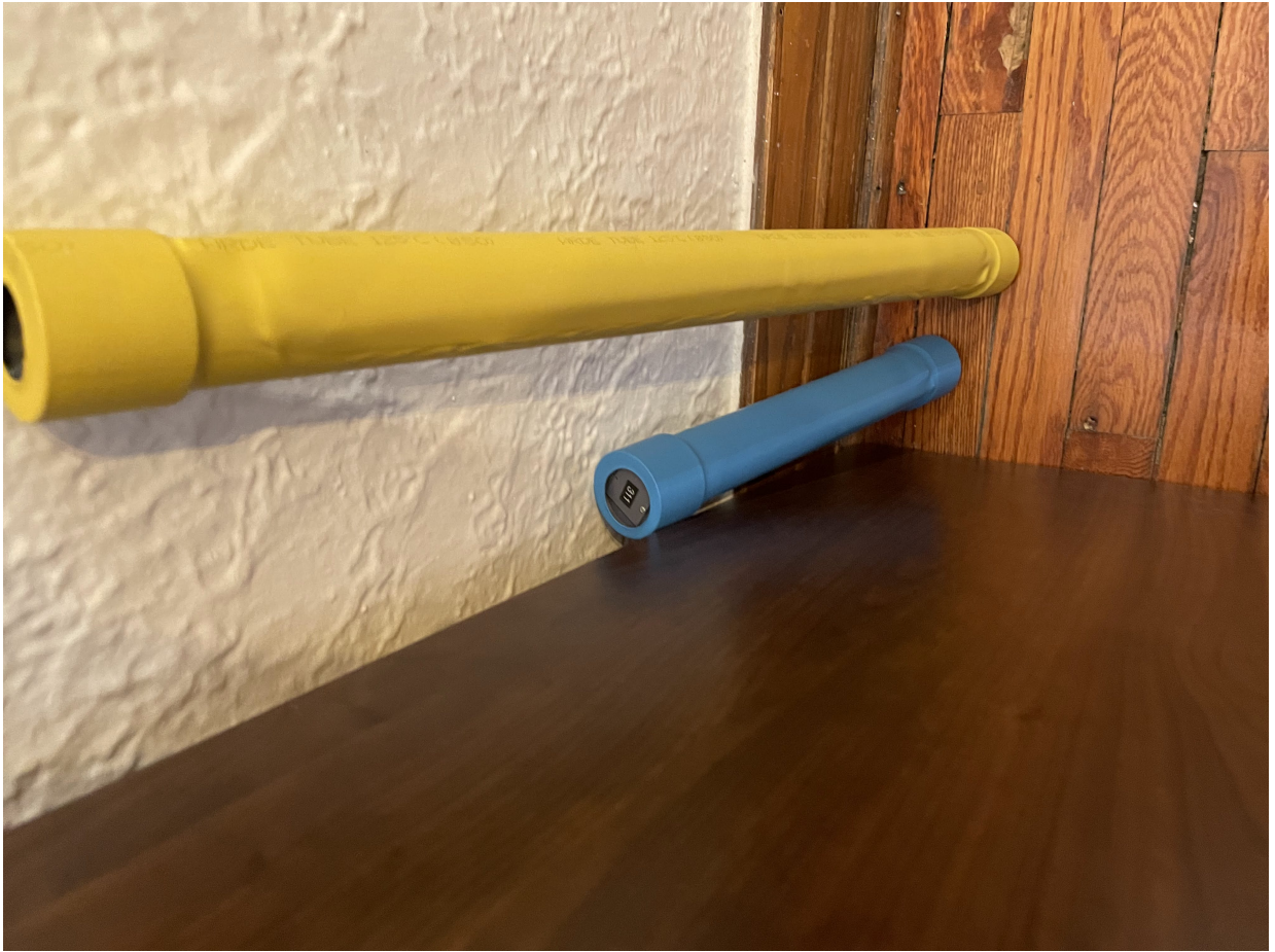
Fig. 2.1 A sopranino and soprano T-Stick.
