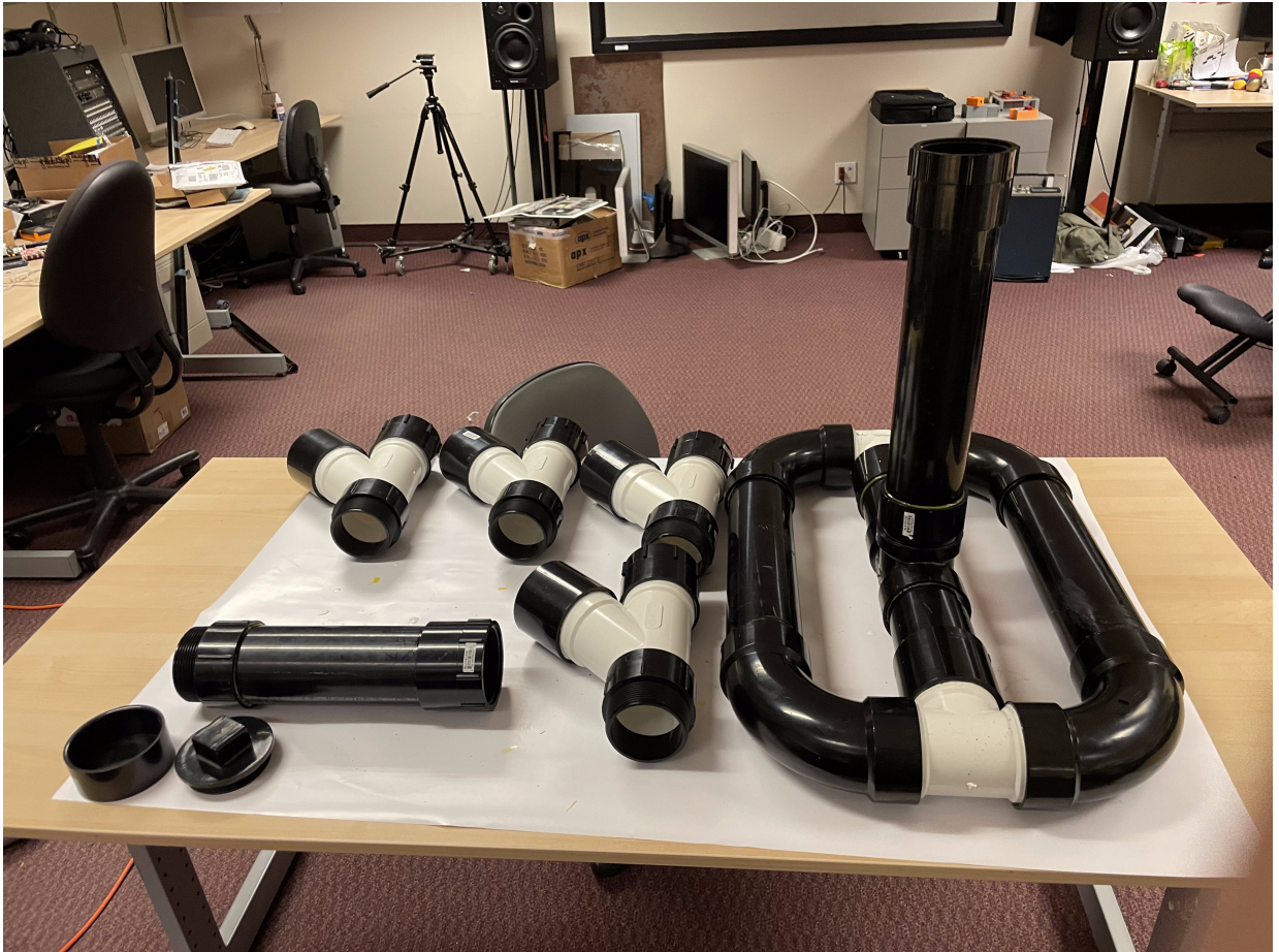
Fig. 3.2 The second T-Tree 1.0, deconstructed into its modular components. Clockwise from top-left: the four branches, the base, and the brain. Threaded PVC pipe allows these components to be unscrewed for transport and storage.
