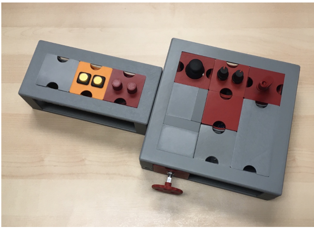
Figure 3: Probatio assembled with color-coded blocks. Red blocks output continuous sensor data, orange blocks output discrete sensor data, and grey blocks don't output data but provide structural support.
