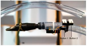
is supported by the performer's left hand, reproducing a saxophonist's hand position, which aims to maintain instrumental technique and to minimize fatigue while holding the eTube directly in one's hand (see Figure 3). A custom 3D printed mouthpiece adapter designed by Cusson ensures the mouthpiece is securely connected to the eTube. The parametric 3D plan is adaptable for other purposes and allows the parts to be adjusted for various-sized mouthpieces and tube diameters, promoting versatility.
