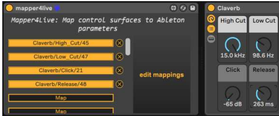
Fig. 4.4 The Mapper4Live plugin interface. Parameters from the Claverb instrument in Ableton Live are exposed on the libmapper network where gestural controllers can modulate their values in real time.
