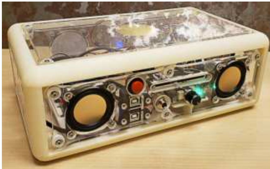
Fig. 3.1 The Tapbox, showing the Top panel with its piezo sensor and the front control panel with speakers, originally presented in (Sullivan, 2021).
