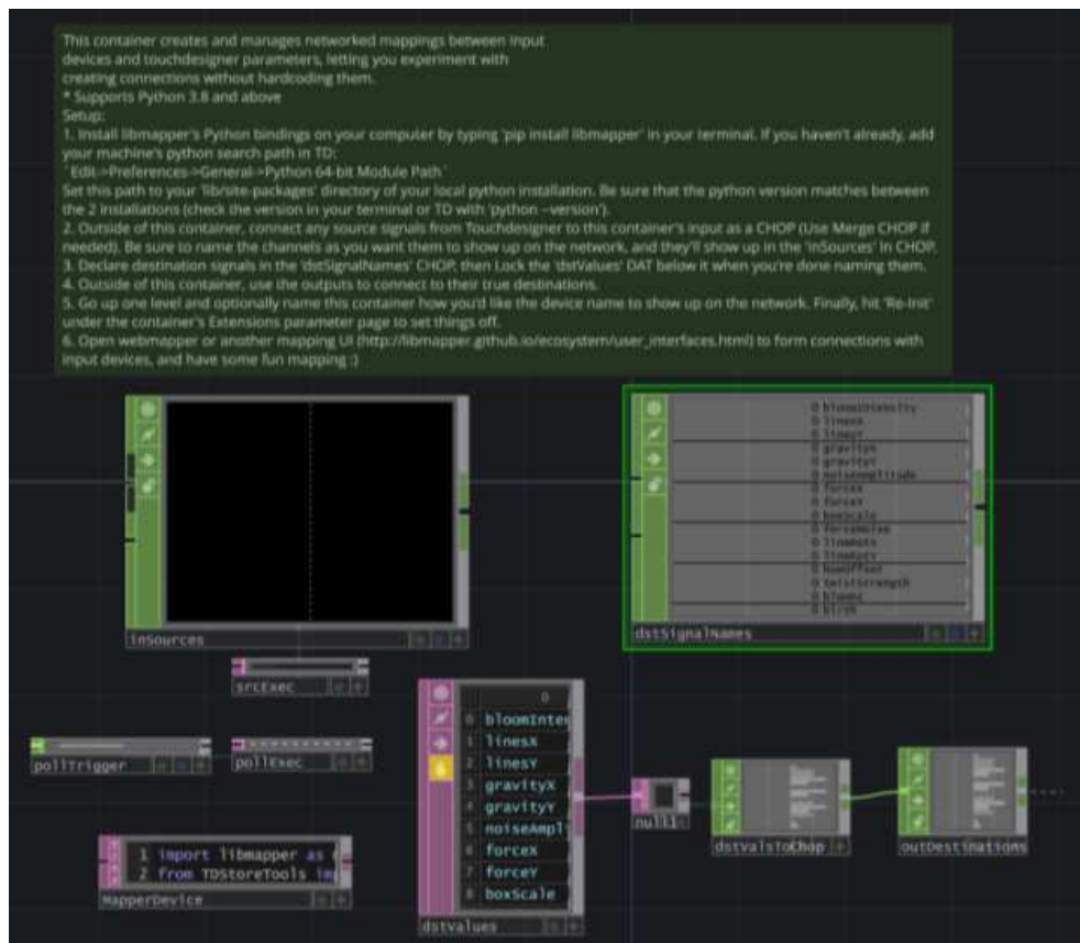
Fig. 4.5 Internals of the Mapper4TD container, showing its inline setup and usage instructions at the top, components for source signals on the left (InSources), destination signals on the right (dstSignalNames) and a libmapper device written in Python that manages signal networking in the bottom left (MapperDevice).
