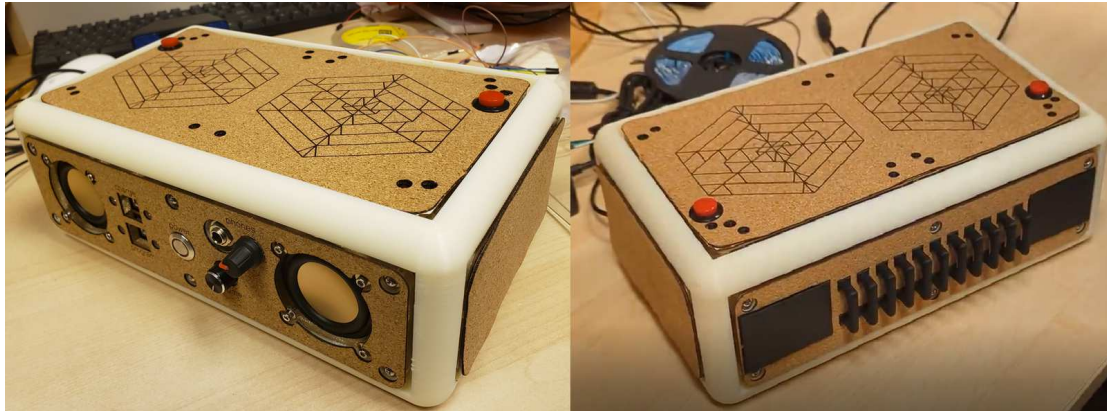
Fig. 3.2 The Slapbox design. Left: Top and front speaker/auxiliary control panels. Right: Top and guiro side. Note the (red) buttons and LED positions in the Top panel.
