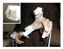
Figure 3. The gesture device uses *flock of birds* sensors with 4 *birds* (receivers). The *birds* are fixed on the thumb and the index of each hand so that no motion is possible between the *birds* and the fingertips. Switches are fixed on each fingertip and can be used like a mouse click button.
