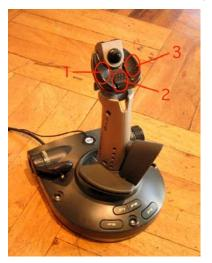
Figure 3: The Saitek Cyborg 3D joystick has 13 buttons and 4 continuous controllers. The three buttons on the top, labeled 1 to 3, can be used to route the continuous controller values to different destinations.
