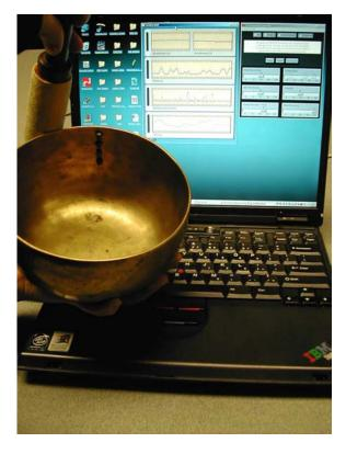
Figure 3: The HyperPuja stick in performance. The laptop screen shows the sensor data display on the left and the sound synthesis GUI on the right.
