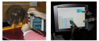
Figure 6. The optical instrument and its digital emulator's interface. The emulator proposes the same control than the real instrument, where the user moves a light in front of the disk and a filter between the disk and the photocell.
