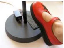
Figure 23. Foot Pressure Sensor
