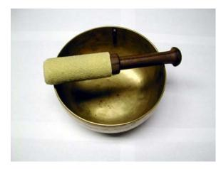
Figure 2: The HyperPuja stick with a Tibetan singing bowl. The magnet for the hall effect sensors can be seen inside the bowl.
