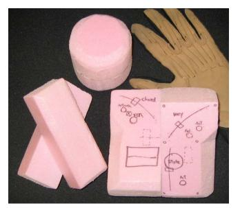
Figure 5. Foam mockups for initial instrument design. The glove is placed for size reference.
