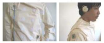
Figure 9: Testing jacket. Left: multiple sensor placement options; Right: user wearing headphones and sensor
