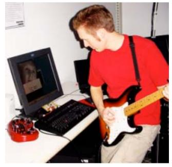
Figure 1: The author using the system. The IR camera is just beneath the monitor, and the effects processor is on the left.
