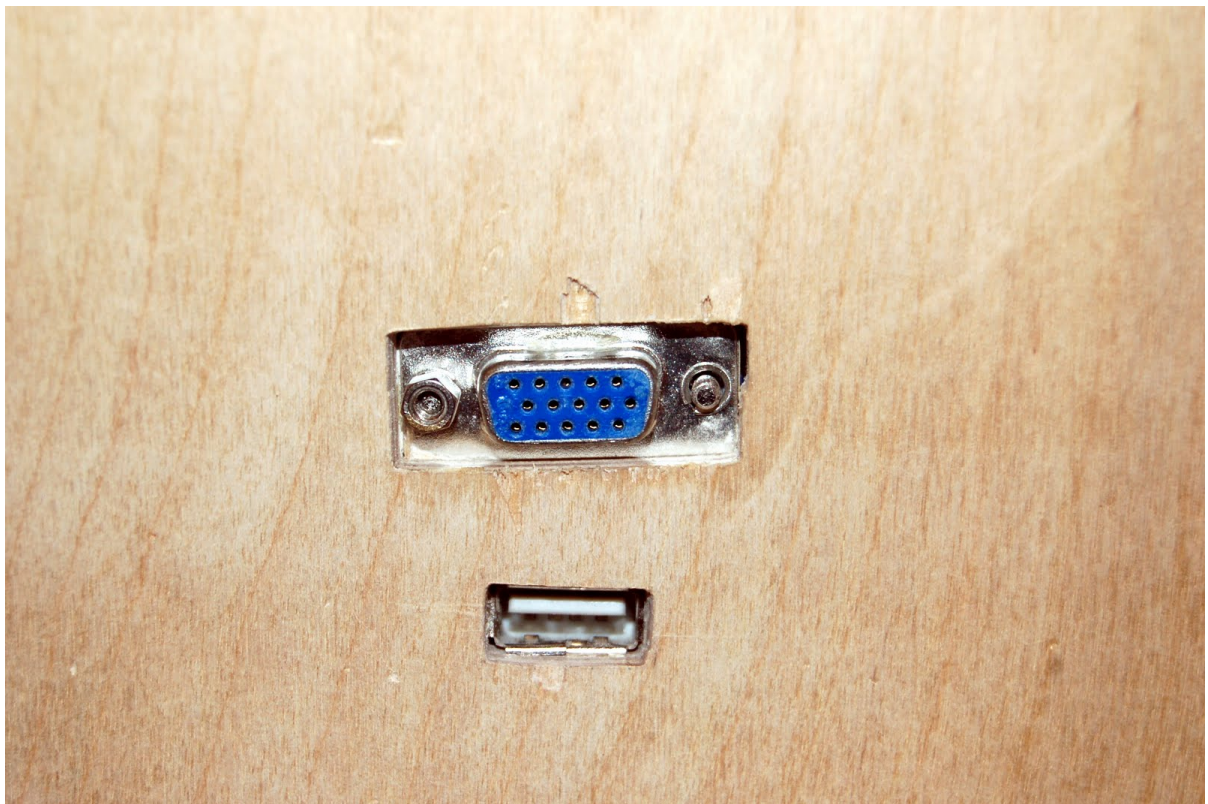
Fig. 2.13 The VGA connector for the projector, and the USB connector of the webcam
