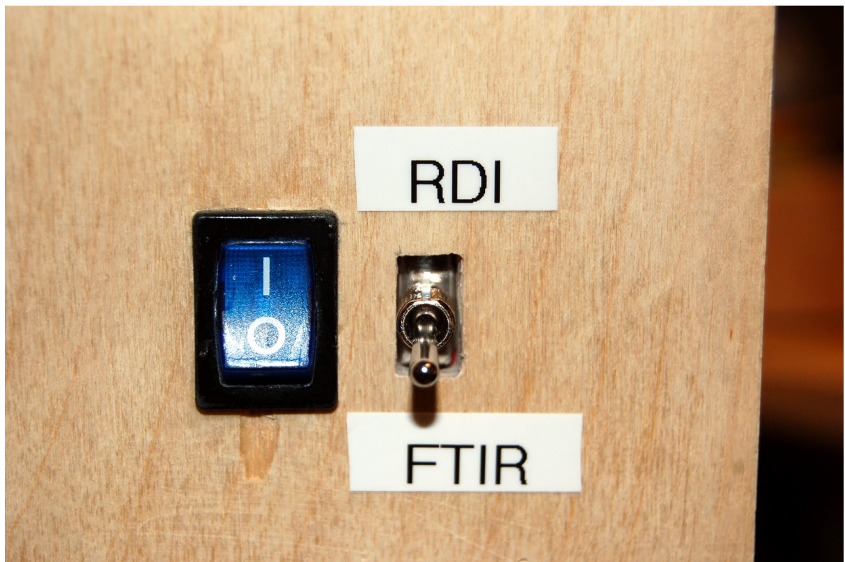
Fig. 2.12 The switch that allows the user to change between FTIR and RDI
